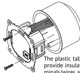
The plastic tab must be in place to provide insulation between the terminals/wires and the mounting screw.
